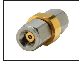
33WW50 Precision W1 Male to W1 Male Adapter, DC to 110 GHz
